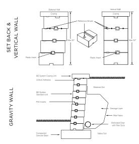
Maximum height for vertical Installation: 27-31.5" (Under optimum conditions) Quarry Wall has a set back of ¼" per course.
