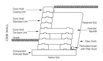
Cross sections are examples and must not be used for construction.
