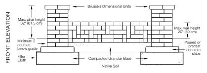
All joints must be adhered with Concrete Adhesive. Base preparation may vary according to soil and climate conditions.
