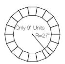
To enlarge the radius for planters and walls, simply 'gap' the back to make the desire radius. (You will not see the gaps because they are against the backfill.) Be sure to use filter fabric between the wall and the backfill. (See Tech Guide for complete instructions.)
