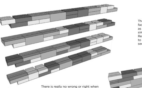
The easiest way to construct a random faced wall is to build them in linear clusters as shown here to the left. This is the simplest way to keep track of the pattern. Remember, the units are totally reversible to alternate between straight and curved sections in the wall.
