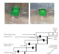
For setback application - Place device perpendicular to channel with round section facing the back of the unit
